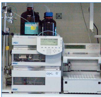
Fig. 1: PSS SECcurity GPC/SEC system with manual injector and fraction collector (courtesy of H.Thijs, Eindhoven University of Technology).
