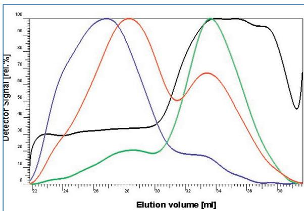
Fig 1: elugram with multi detection of an ethylene-vinyl acetate copolymer
